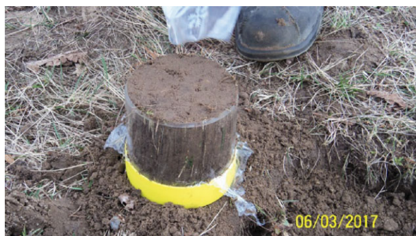
Figure 4. Undisturbed soil sample with 12 cm diameter.
