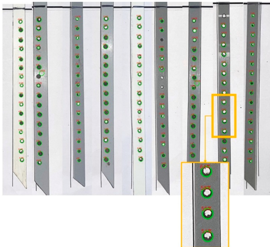
Fig. 8. Example outputs of the automated pipeline overlaid on bait-lamina strips. Each column represents a single strip, showing detected hole locations (outlined circles) and assigned feeding-intensity labels.
