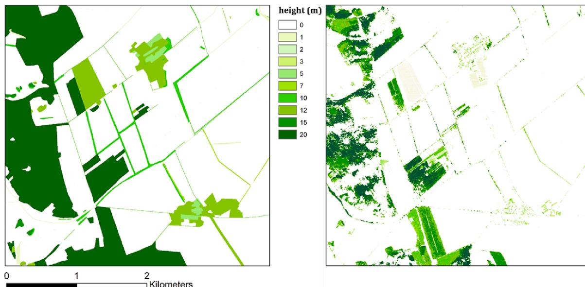
Fig. 4. Section of the landscape elements map, left: assigned heights from the biotope mapping; right: measured heights by laser scanning.
