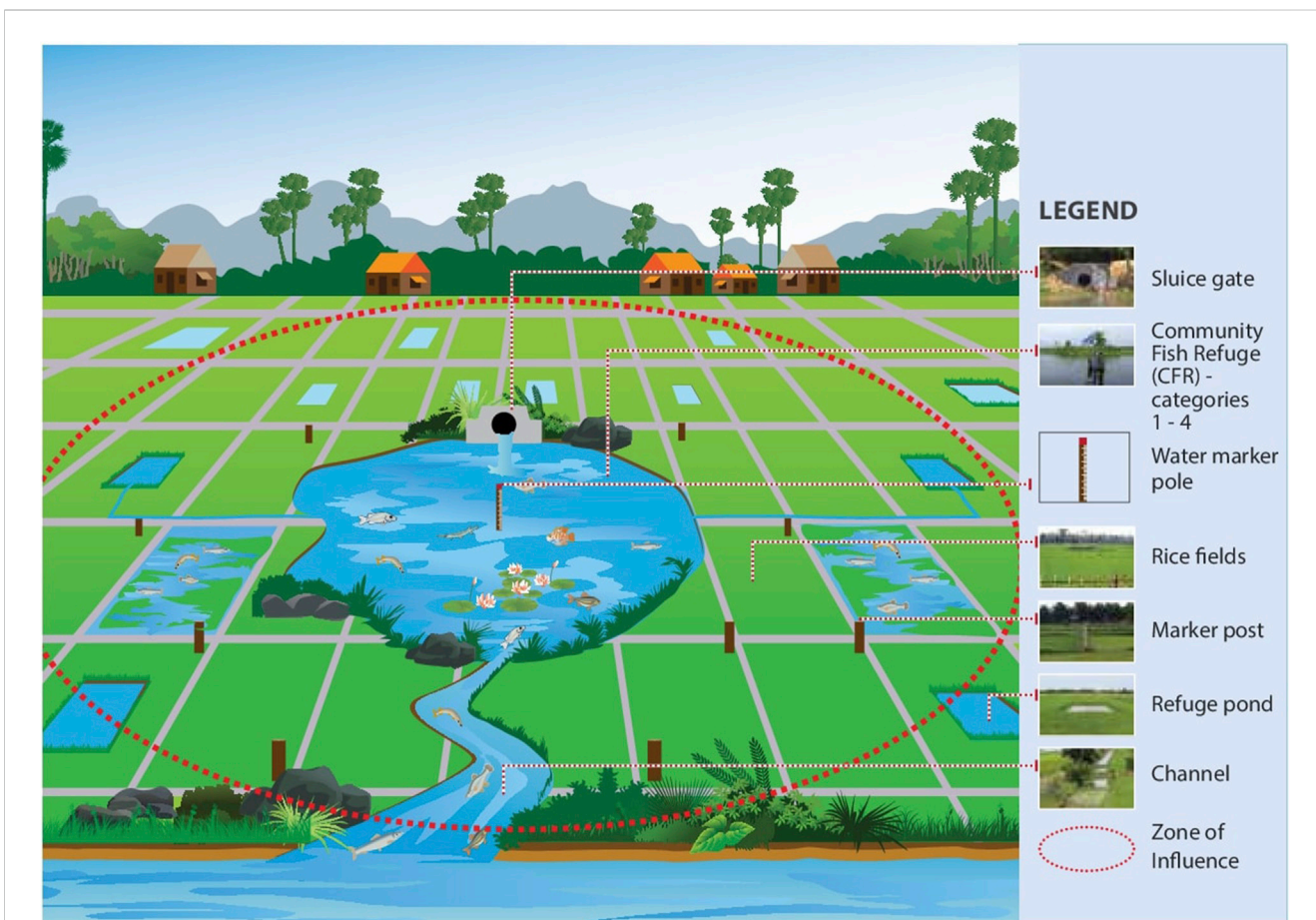
FIGURE 1 Main physical components of the Community Fish Refuge system source: Kim et al., 2019.
