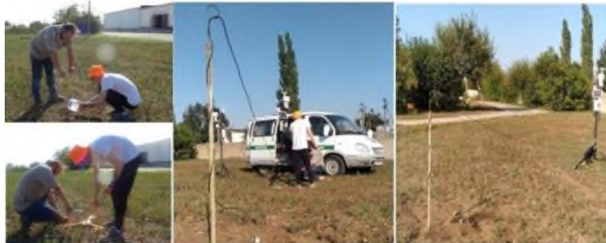
**Figure 2.** Installing the rod sensor in the soil.
